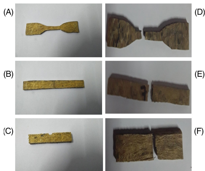
FIGURE 2 Test samples before fracture for: (A) tensile test, (B) flexural test, and (C) impact test; after fracture for (D) tensile test, (E) flexural test, and (F) impact test [Color figure can be viewed at wileyonlinelibrary.com ]
