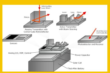
In the present day scenario of **Embedded applications in Wireless** Technologies Smart Dust Mote sensors is exploring the limits of autonomous sensing and communication by packing entire system into cubic millimeter at a relatively low cost. volumetric These constraints correspond to energy constraints
